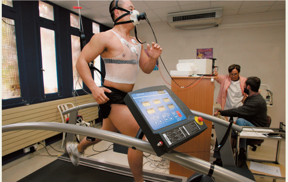
A man exercises on a treadmill wearing a device that measures his rate of O_2 consumption. His speed can be controlled by adjusting the speed of the treadmill.
