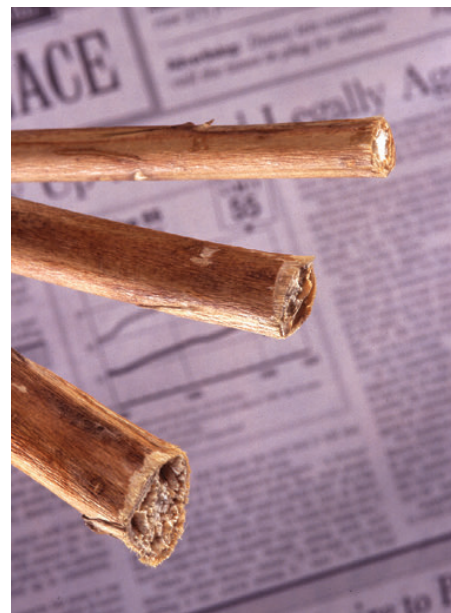
FIGURE 24.17 Kenaf Stems The stem of kenaf plants is rich in long phloem fibers. Their low lignin content makes the fibers attractive for making paper as well as other products. Paper derived from kenaf fibers has been used for printing newspapers.
